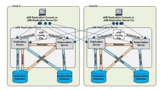
In the figure, two Postgres installations are running on two networked hosts, each with its own Replication Server installation. Each host is running a publication server and a subscription server.
